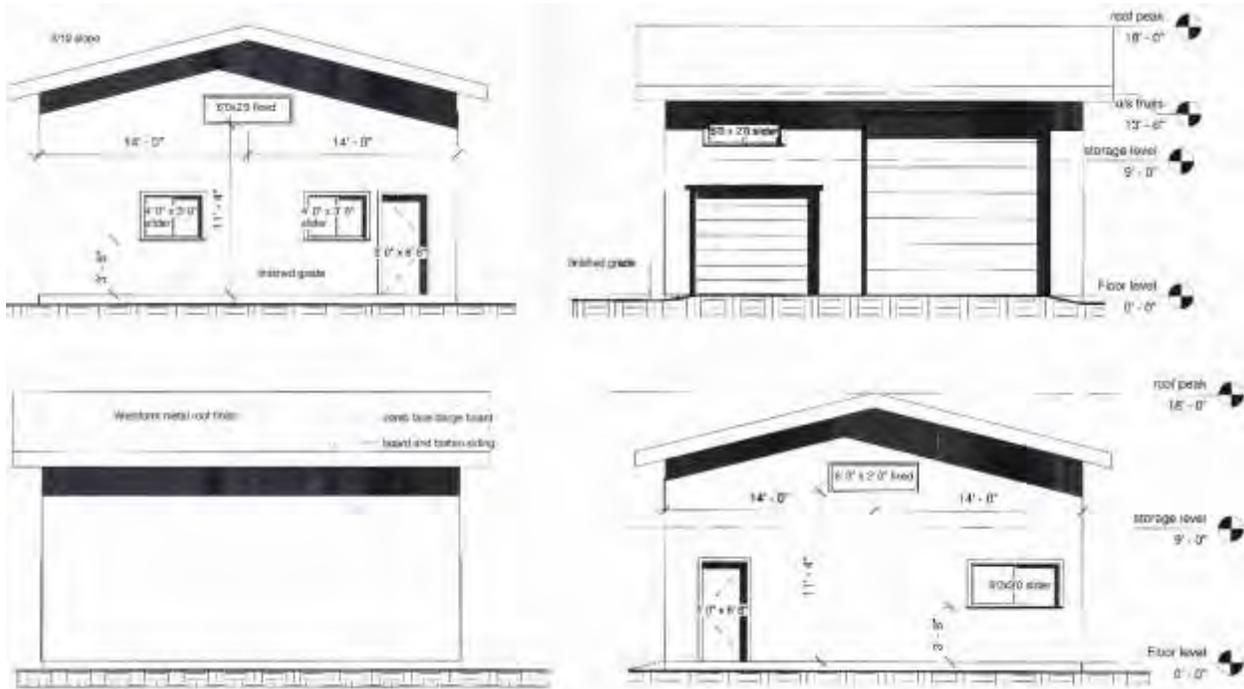
Figure 4: Elevation Drawings of the Proposed Accessory Building
